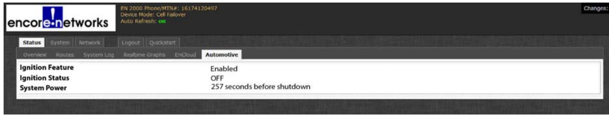
Figure D-4. Automotive EN-2000 System Power Status Screen: Countdown to Power Shutdown
