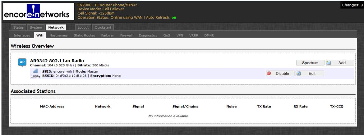
This screen provides basic information about the card's wireless specifications; it displays the MAC ID and supported versions of 802.11 (in [Figure 6-17](#), 802.11an). If the wireless card has already been configured, the display also lists the card's mode and related specifications.
