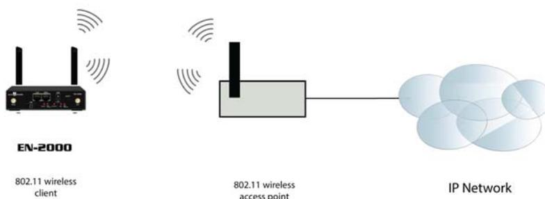
To configure the wireless card as a client, you must first identify the wireless access point that the wireless card will connect to. That access point must support the type of 802.11 wireless transmission that the EN-2000 supports (802.11a, 802.11n, or combined support for 802.11a+n). You must also know the password (and other credentials, if applicable) to log on to that access point.
