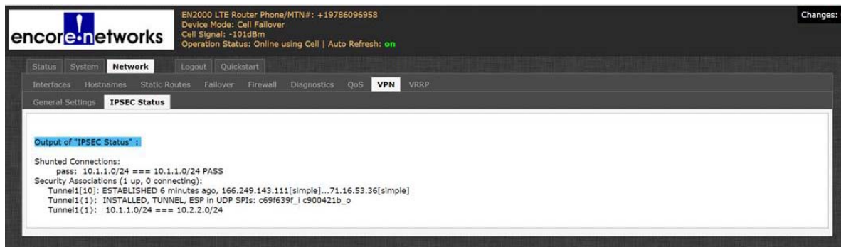
Figure 12-6. Status of IPsec VPN Tunnels
