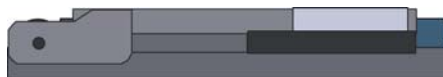
Figure 2-19. Closed SIM Socket with New SIM (Side View, Door Not Yet Locked)
