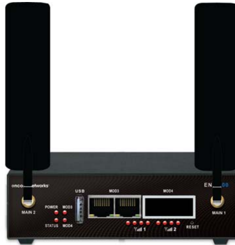
Figure 2-25. Front of EN-4000 Chassis, with Antennas
