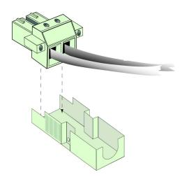
Figure 2-6. Cabled DC Power Connector and Bottom Section of Shell
