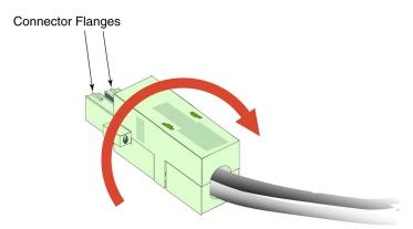
Figure 2-9. Rotate DC Shell Assembly 180 Degrees around Axis of Power Cable
