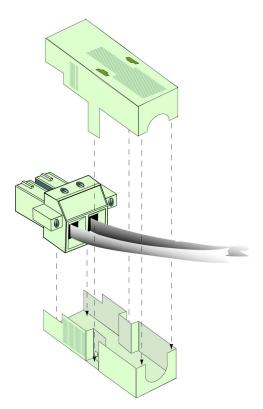
Figure 2-7. Top Section of Shell above Cabled DC Power Connector and Bottom Section
