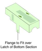
Figure 2-1. Top Section of Connector Shell
