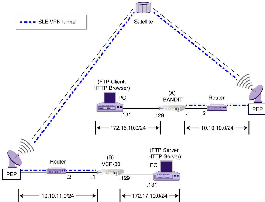
Figure 9. Sample Satellite Network Configuration Using Encore Networks' SLE VPN
