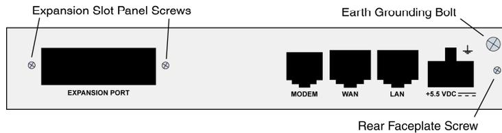
Figure 4. Original BANDIT Chassis, Rear
